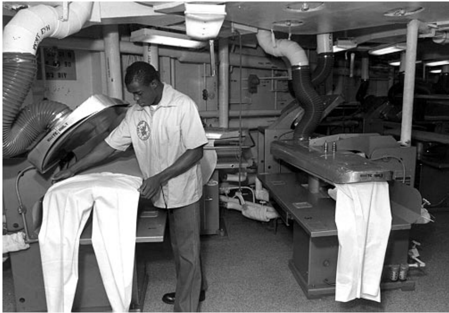
Figure 5-34.-Laundry press single operator station.
